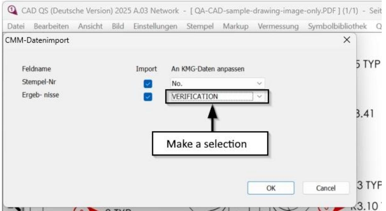
3. After the import, the measured values (results) and pass/fail are also displayed in the table. The measurements that are outside the tolerance are highlighted in red in the drawing.
